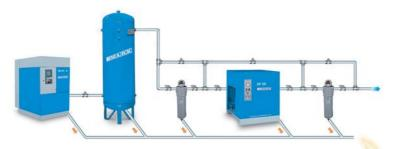
As an example, if a compression system with a refrigerant dryer with a capacity of 20 m³/min, 10 bar were to operate at 60% full load, two shifts a day, for 220 days/year, at a room temperature of 25 °C and 70% relative humidity, its condensate production would be about 39,000 litres/year.
